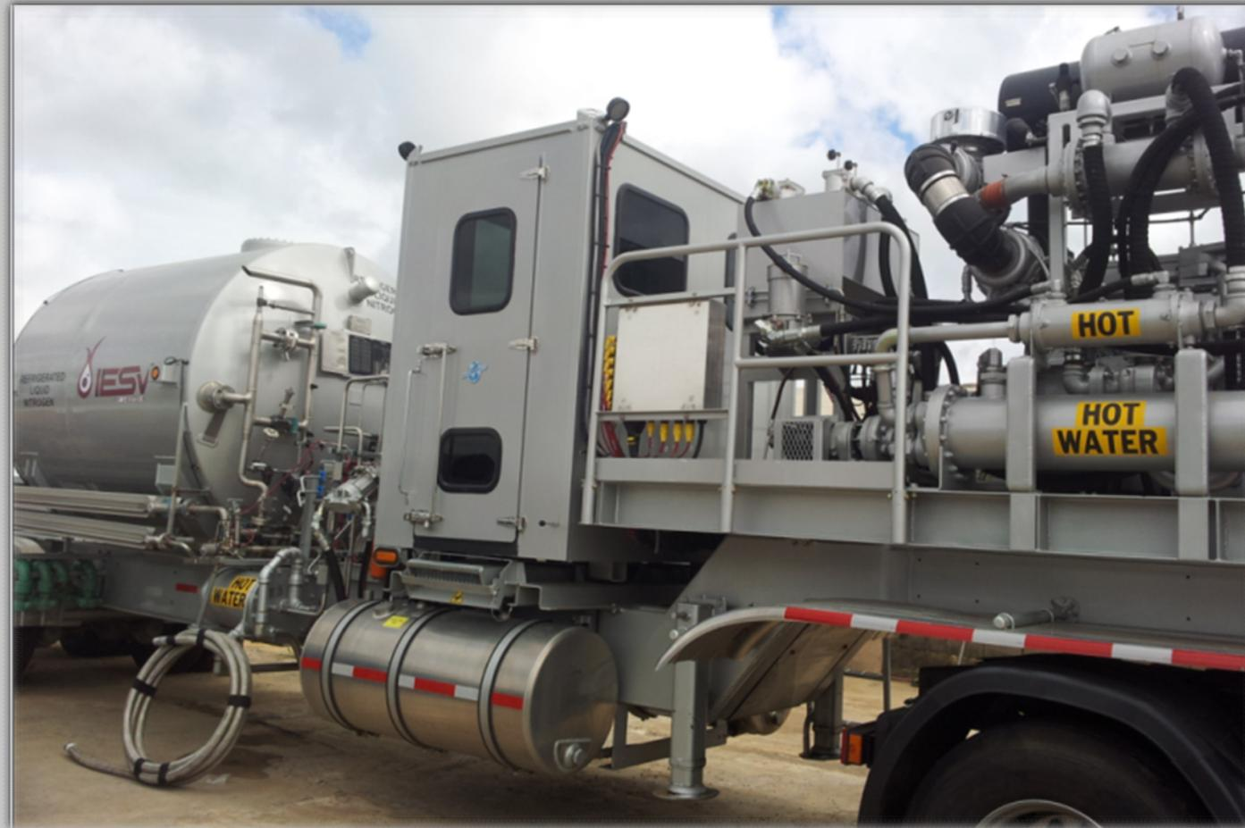
**UNIDAD DE BOMBEO DE NITROGENO, MODELO NT-181-NF, 180K SCFH TRAILER-MOUNTED, NON-FIRED NITROGEN VAPORIZER AND PUMP – GENERATION 2.**
